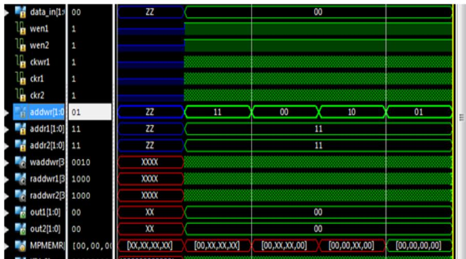
Fig. 4 Memory4x2 simulation result
