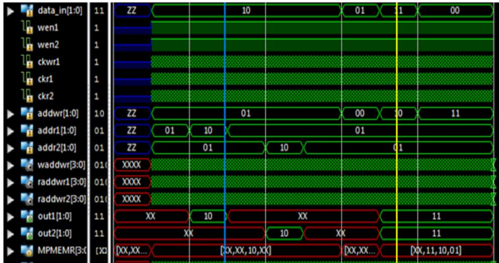
Fig. 3 Memory4x2 simulation result
