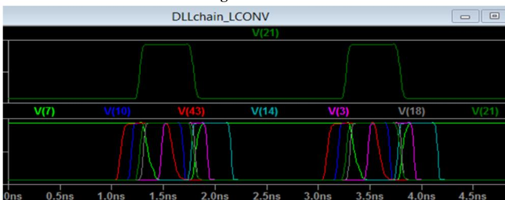
Fig. 2 Time shifting of generated frequency to match input waveform
